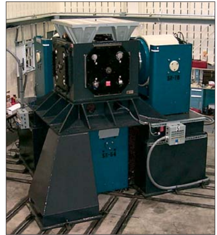
Figure 2. Three 20,000-lb-force shakers for simultaneous testing on three axes.
